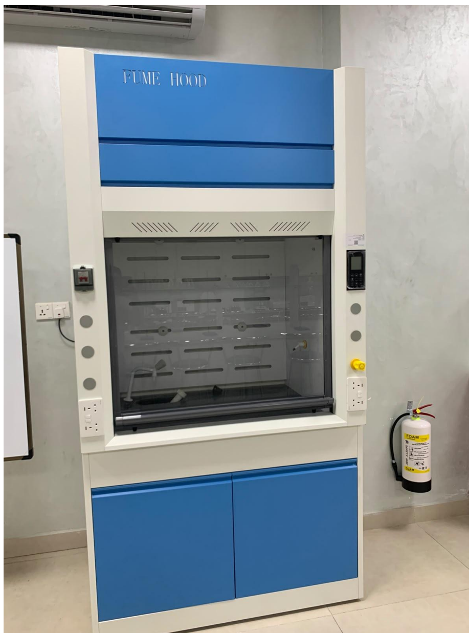
Figure 2.1.6f: Front view of the heavy-duty Fume Hood cabinet with sash glass, digital exhaust controls, electrical outlets, and adjacent foam fire extinguisher.
